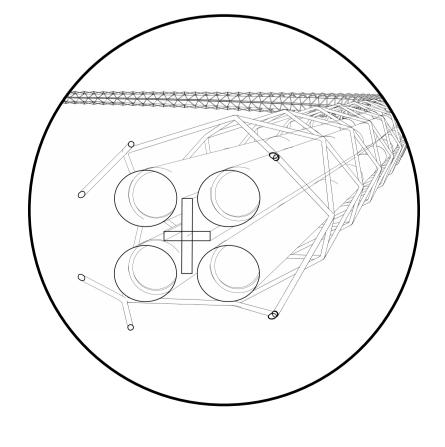
Transportation path to increase mobility for humans and resources transport during early stage of habitation. The path consist of 4 transparent vacuum tubes for 2 way travel. High velocity trains will be moved using magnetic propulsion inside the vacuum tubes. The path structure will be supported by a metal exoskeleton structure.
